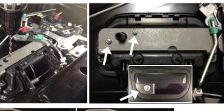
**STEP 3** - Using the bracket holes as a template drill the two 3/16" (or 5mm) holes and one 1/2" (or 12mm) hole. Insert the lock assembly from the front of the bezel inserting the shaft through the 1/2" hole and aligning the two mounting holes on the bezel with the mounting bracket. Insert the 2 supplied 8–32 x 1 1/2" screws through the mounting bracket in to the bezel. Tighten the screws. DO NOT OVER TIGHTEN. IF LOCK ASSEMBLEY BINDS LOOSEN SCREWS UNTIL THE KEY MOVES FREELY!
