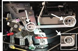
**STEP 5** - Install the crank rod assembly by hooking the slotted end onto the bolt linkage and the square hole to the end of the lock assembly shaft. Insert the 1/4" x 20 x 2" screw into the shaft and tighten.
