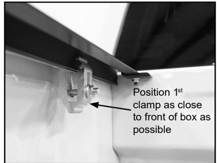
**NOTE:** Images below illustrate clamping options. **Option A** depicts standard clamping orientation lower on the side rail. **Option B** depicts alternate clamping orientation with half of clamp assembly rotated 180° to provide better grip at top of side rail.
