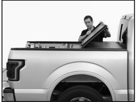
C. Always ensure all latches and hooks fully engage side rails. Close tailgate.
