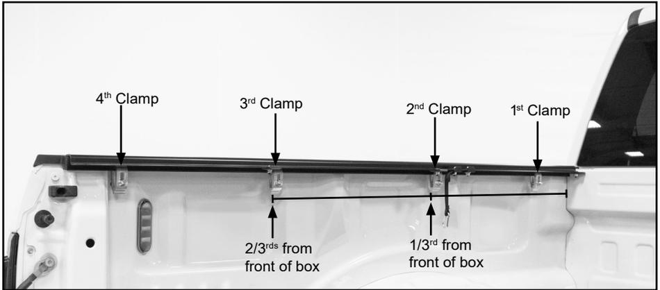
**NOTE:** For trucks with electric tailgates, typically side rail must be installed slightly higher to eliminate interference.
