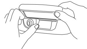
Lift the handle all the way up and insert the lock assembly into the pocket under it. Tilt it up so that the two hooks slide into the cutouts for the handle arms. The top edge of the lock assembly should clear the bottom edge of the handle. Push it in evenly and forcefully until the hooks snap into place. NOTE: If the handle doesn't clear, remove the tailgate access panel and release the rods to get additional lift.
