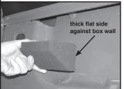
a) At front corner (behind cab) use 1 small foam wedge positioned as shown. Thick side against box wall.
