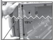
a) At tailgate, measure from top of box down to 19½" and make small mark. Repeat on other side.
