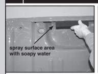
a) At rear of box, spray with soapy water for easier installation. Place long foam up under box lip. (thick side against box wall)
