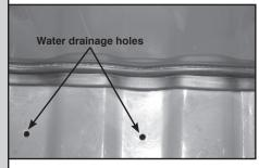
a) Water drainage holes on floor behind cab. b) Black nylon wall plugs. Seal if desired Seal with silicon if desired.
