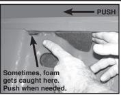
b) Compress foam and push while guiding lead end into cavity.
