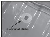
floor behind cab. Wipe with alcohol. Apply clear seal sticker over hole.
