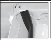
a) At top of box, by tailgate (makes sure area is still clean) start applying TrailSeal 1" back as shown above.
