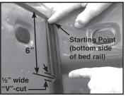
Note: Starting point for ACCESS cover shown (underside of bed rail) other applications may need to be started higher.
