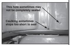
c) Sometimes hole is not sealed on floor and OEM caulking sometimes stops short at end of box. Seal with silicon if desired.
