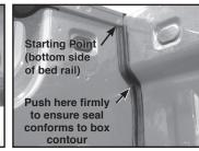
c) Peel adhesive protector as needed from both legs. Begin adhering seal to inside corner where box walls meet. **Push** firmly in center of seal following contour of box down to floor.
