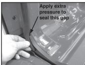
c) At the bottom, curve trailseal under the "L" seal as shown.
