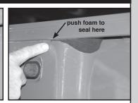
d) Continue pushing foam into cavity until it fills small opening. Then pull back slightly to fill large cavity.
