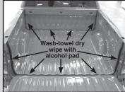
Thoroughly clean inside area of box (where seal adheres) with mild soapy water. Towel dry. Wipe with alcohol pad (save 2nd alcohol pad for later). See above.
