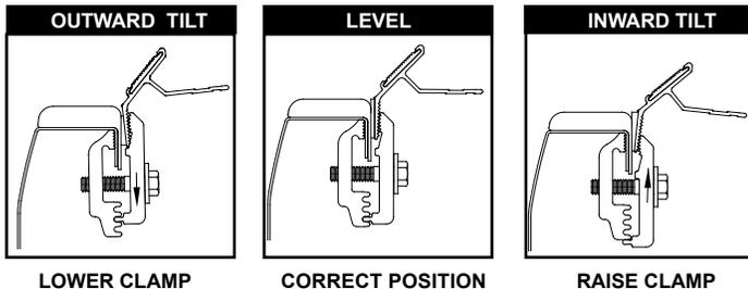
**NOTE:** Clamp configurations shown above are for reference only, and are not intended to be standard for all pickups.
