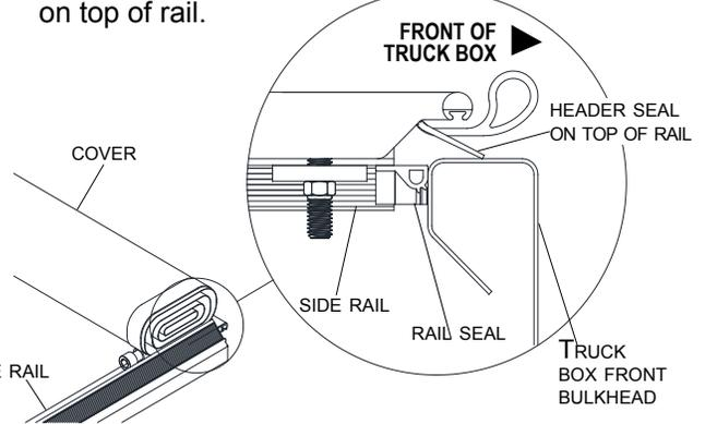
**STEP 5:** Tighten bolts but do not over tighten. Header must be free to slide.
