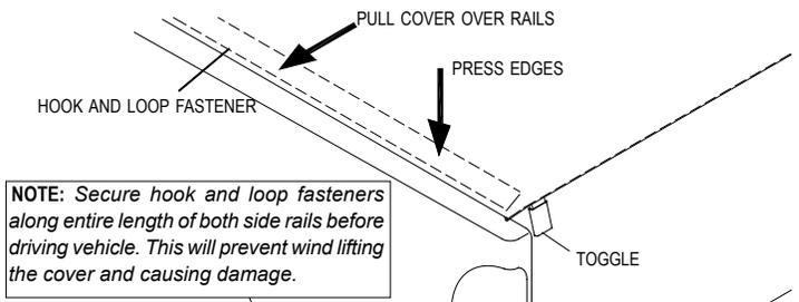
**STEP 8:** To release cover, Trigger pull rear release toggle. Start rolling cover toward cab making sure both sides of cover roll evenly. For best results leave unrolled portion of cover attached to the hook and loop fasteners while opening.
