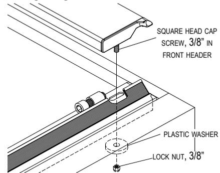
**STEP 4:** Set cover assembly behind cab with header seal on top of rail.
