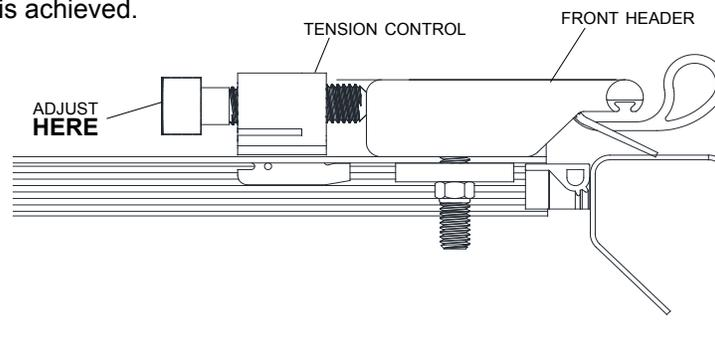
**NOTE:** Adjust tension in small increments. Slight adjustments yield significant results.
