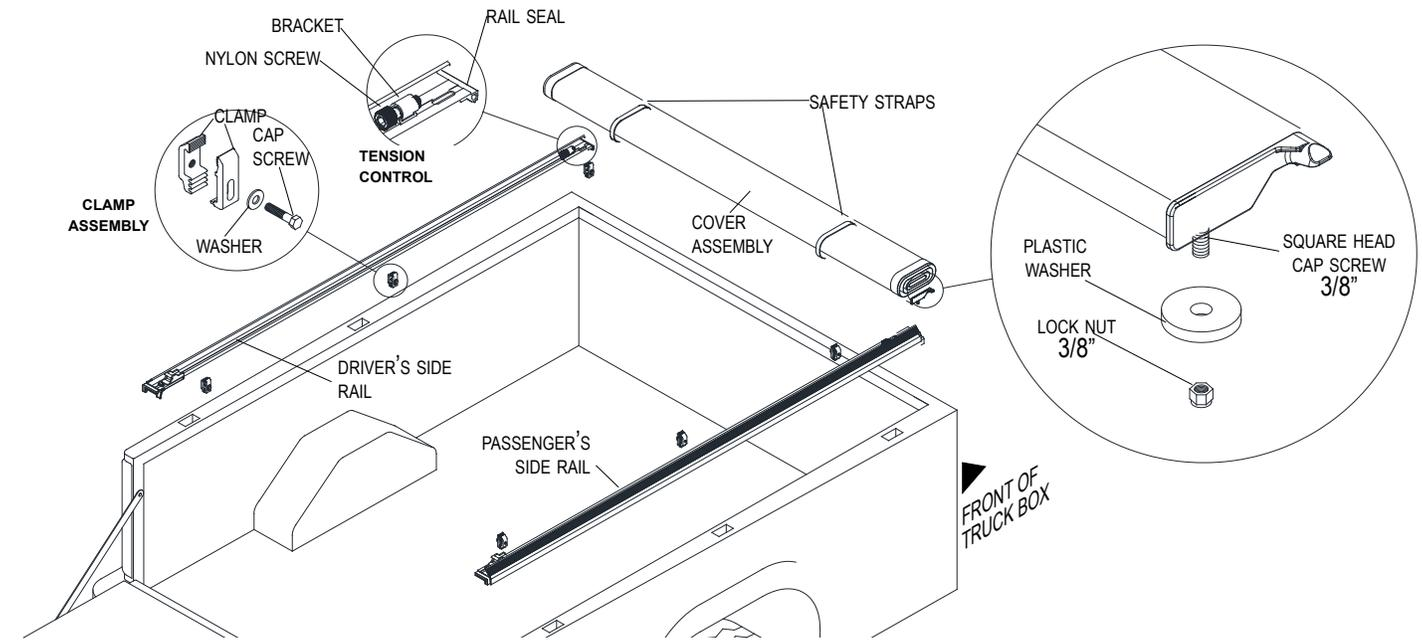
**STEP 1:** Place side rails on truck box compressing front rail seal slightly. Rails must be flush with box rail and level with each other. Starting at tailgate, evenly space 3 clamps along each side rail, leaving about 8" on each end.
