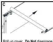
Roll up cover. Do Not disengage loop and hook fasteners prior to rolling up cover.
